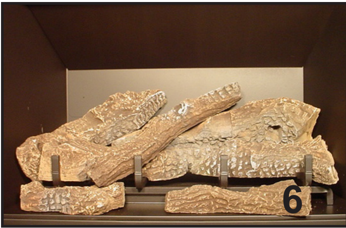
LOG #6 (SRV550-718): Place log #6 on the base on front of the grate as shown.
